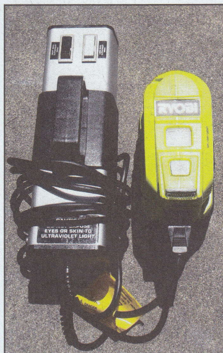
A commercial SW/LW lamp with portable power pack. (Photo by John Norman.)
