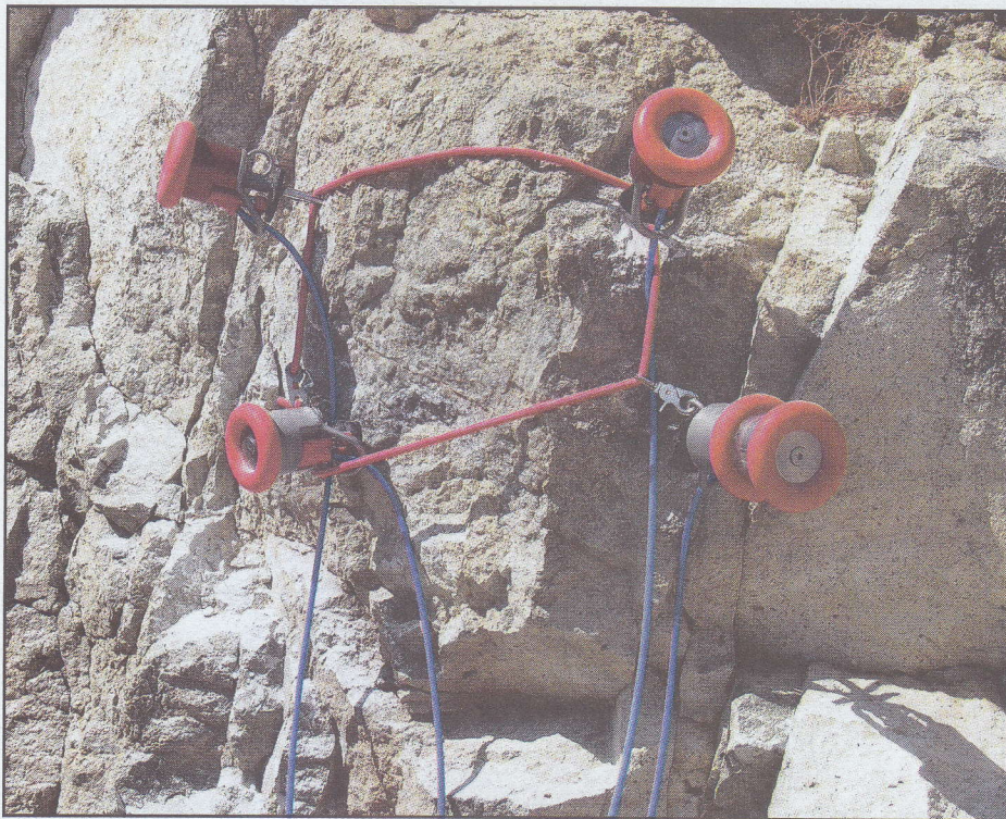
A four-blasting head wedge pattern waiting to be anchored in and fired. The holes are angled in like a wedge to give the force of the blast space to break to.
