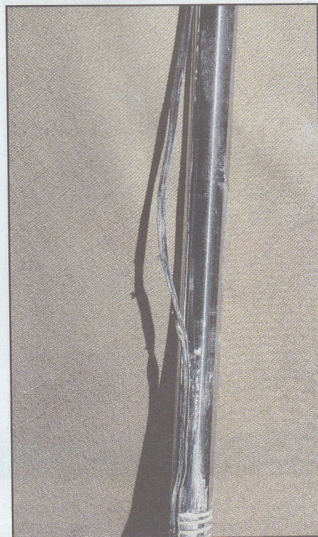
Betty places the blaster head in the hole. It should slide into place without twisting to avoid damaging the electric wires that set off the blast. (Right) cartridge failed to fire. This closeup shows how the wires were damaged due to twisting the head during insertion.
