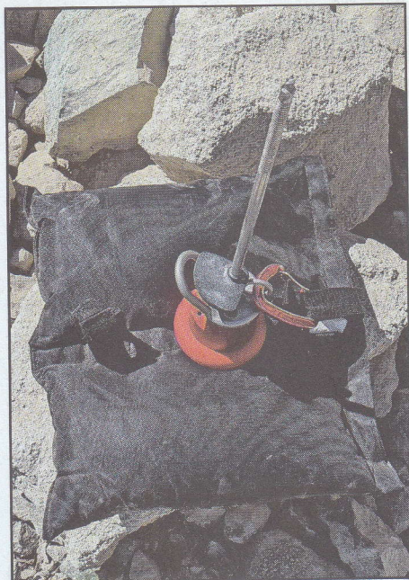
Demonstrating the use of a theatrical sandbag to give blast head weight and hold it down. The sandbag is attached to the blasting head with a climbing carabiner.
